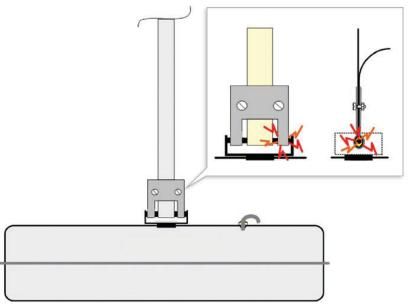
Figure 3. Chemical Safety Board sketch of Float Linkage with front and side view insert where spark likely occurred (in red).
