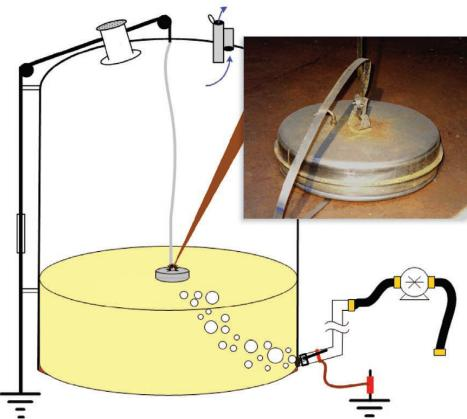
Figure 2. Chemical Safety Board sketch of the 15000 gallon storage tank during filling showing grounding of the tank and transfer line (lower right), but no grounding of float device (with photo insert of float device).
